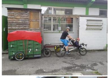
friendly way and without sitting in traffic. CARLA can be combined with almost any regular bicycle or e-bike. Thanks to an integrated mechanical overrun brake, it is possible to carry heavy loads with exceptional safety. Additionally, an electric support can make the Carla even more agile and faster.
